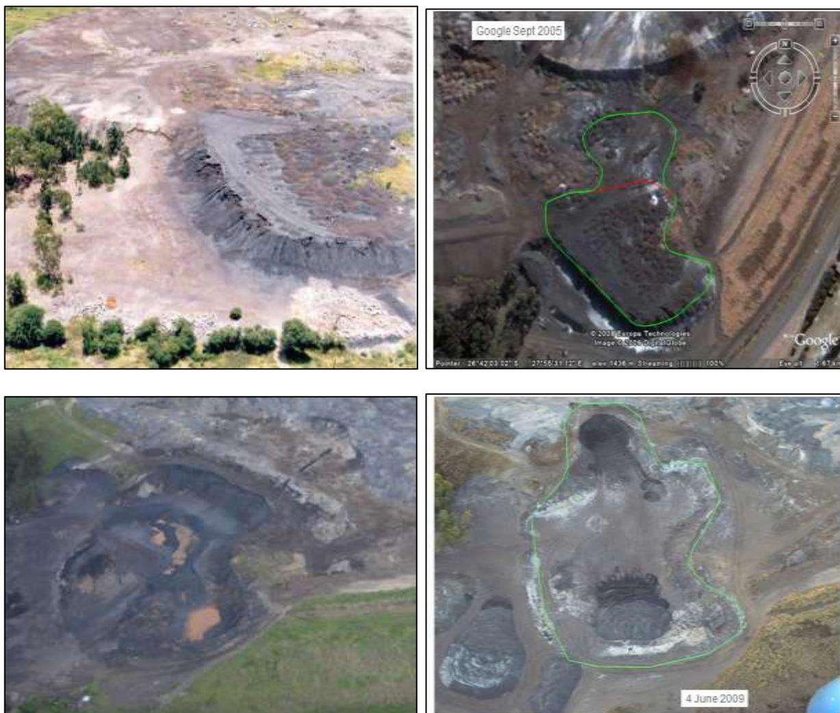
Photo 1 -4 Progressive removal of Magnetite from the Vaal Disposal Site
